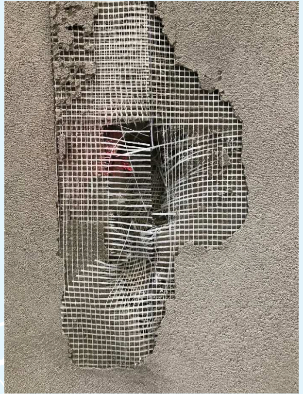
Photographs of the sample after large missile impact test in area C
