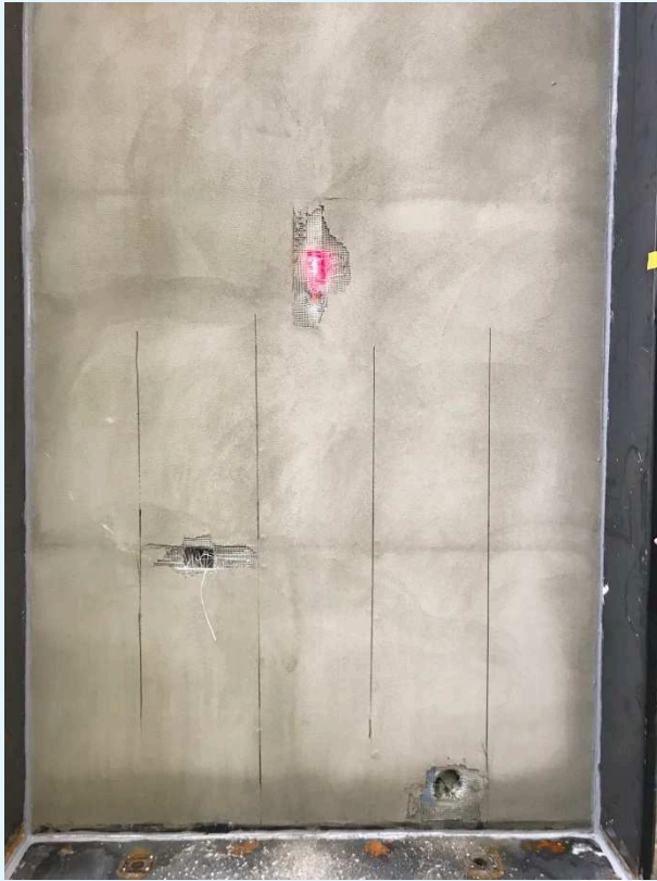
Photographs of the sample after large missile impact test in area C
