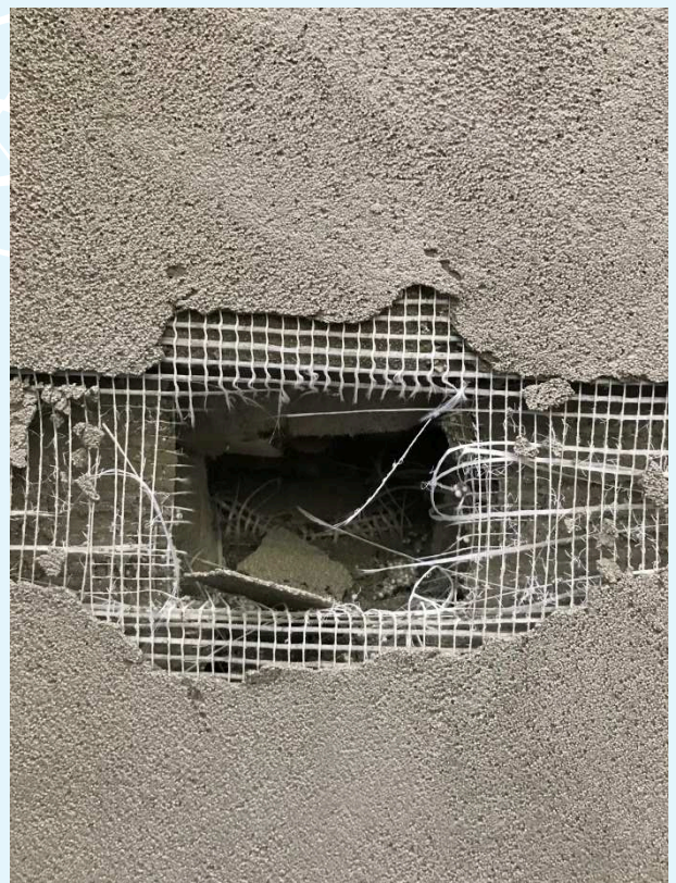
Photographs of the sample after large missile impact test in area B
