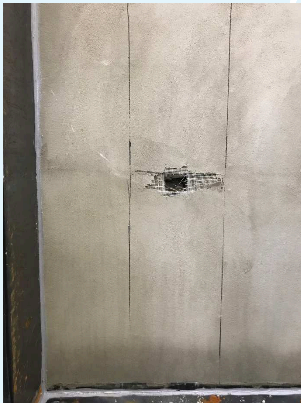
Photographs of the sample after large missile impact test in area B
