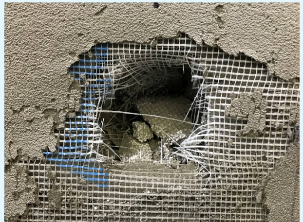
Photographs of the sample after large missile impact test in area A
