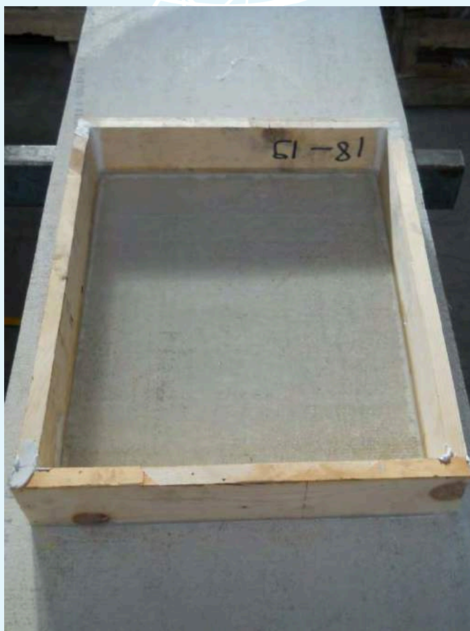
Photo of specimen during the impermeability test
