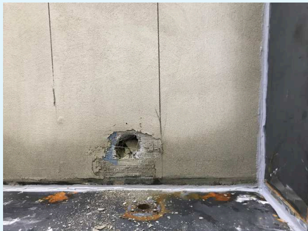
Photographs of the sample after large missile impact test in area A
