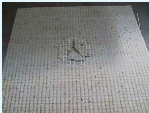
Example of failure with pull-out of screw
